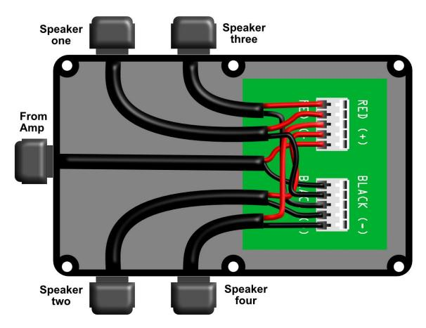
Strip back  $\frac{1}{4}$  to  $\frac{1}{2}$  inch of each wire exposing the core. Use a small screwdriver or similar tool to open each terminal by pushing straight back on the corresponding white tab. This will open the terminal and you can place the stripped end of the wire through.
